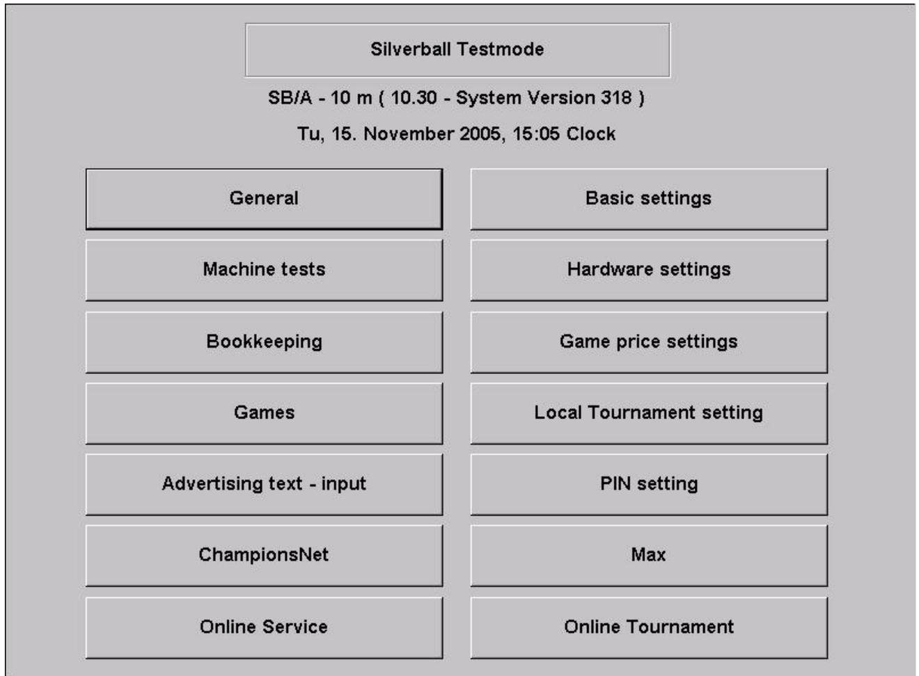
You may make all the machine's relevant settings in the test mode. The precise software version of the **Silverball Strato** and the **dongle version** are shown on the top edge of the screen.
