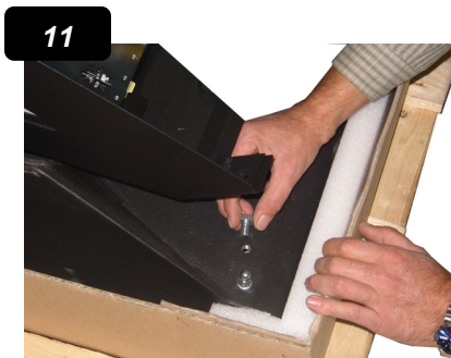
11 Remove the 4 screws from the bottom.
