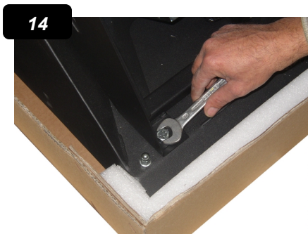
14. Mount the middlepart with the 4 screws on the bottom.
