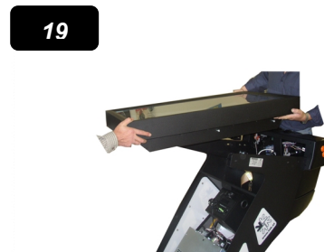
19. Put the Plasma unit in the base-frame. Be careful.
