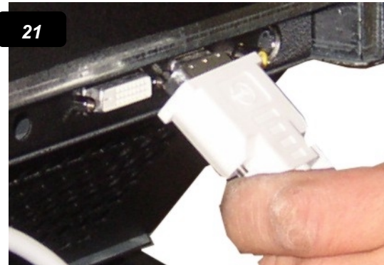
21 Connect the DVI connector.
