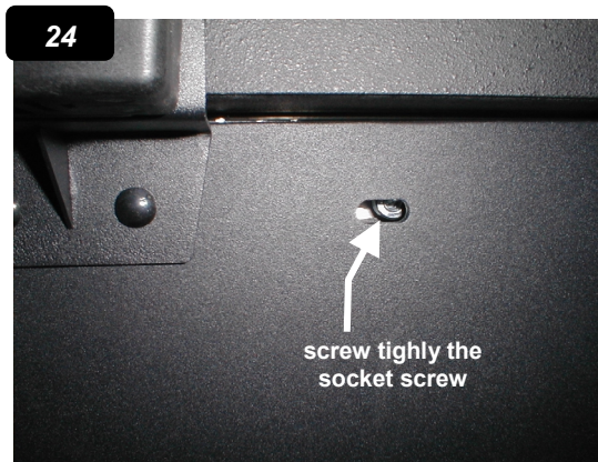
Attention 24. Mount the plasma unit left and right with 2 screws on the base frame. The 4 screws for mounting are fixed in the plasma unit.
