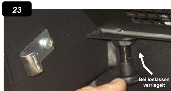
23. The display is now bolted.
