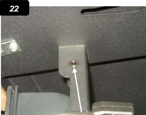
22. Push down the knob to get the plasma into The right position.
