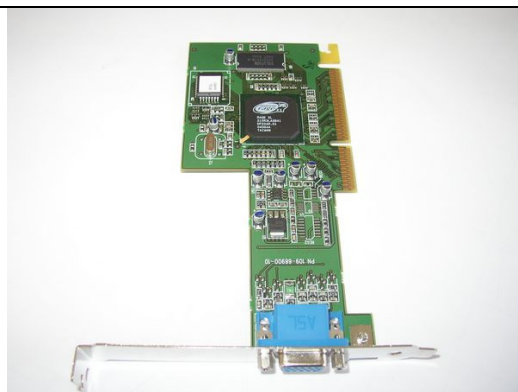
831.200.014 PC Grafikkarte ATI Rage XL AGP ab System 22 (Silverball V7.30, Max Fire V1.11)
