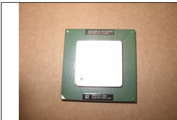
831.000.071 PC CPU Pentium III 1,2 GHz, socket 370 for Virtual Pinball and Max Fire (Video) with QDI Motherboard - 831000044
