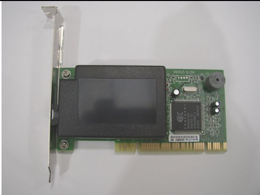
831.800.053 PC Modem PCI intern 56K NEU analog ab System 2 (SILVERBALL V5.5, Max Fire V1.00-V1.18)
