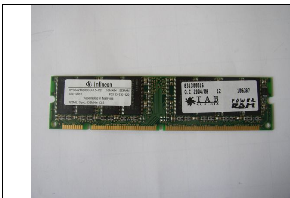
831.300.016 PC RAM 128MB DIMM 168pin - 133MHz
