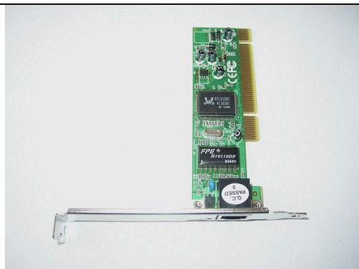
831.800.060 PC Network Card Ethernet 10/100 from System 7 (Silverball V6.03, Max Fire V1.00) and from System 122 (Max Fire Video V1.00, Virtual Pinball V1.10, Virtual Casino V1.07)
