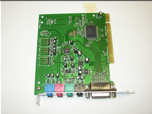
831.200.009 PC Sound Card Creative Lab 128 from System 32 (Max Fire V1.18 and Silverball V9.32)
