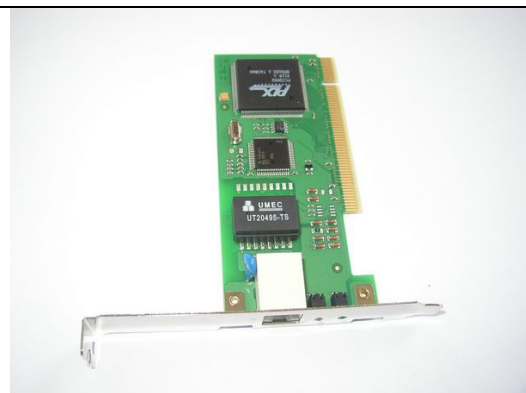
831.800.051 PC Modem PCI Internal ISDN ELSA Microlin from System 16 (Silverball V7.04, Max Fire V1.00-V1.18)
