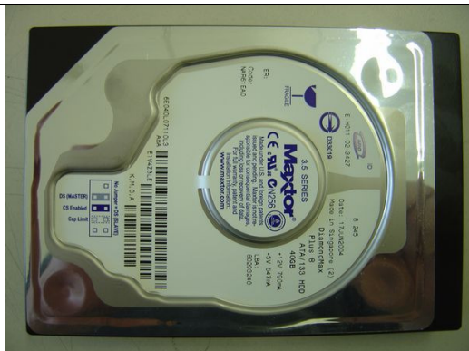
831.000.048 PC HDD 40 GB Adjustable to 32GB Hard disk(40GB, but can also be adjusted to 32GB with "Cap Limit" Jumper) With 32GB it can be applied as an exchange disk for all motherboards that were supplied up to Silverball version 6.30 (all boards before changing to ACORP). Do not use for ACORP and QDI boards!
