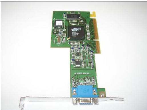
831.200.014 PC Graphic Card ATI Rage XL AGP from System 22 (Silverball V7.30, Max Fire V1.11)
