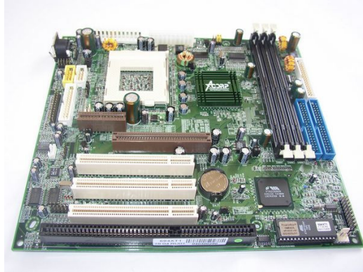
831.000.024 PC Motherboard Acorp 694XT BIOS 46 for 800x600 / BIOS 47 for 640x480 from System 10 (SB V6.30, MF V1.00) and from System 122 (MV V1.00)
