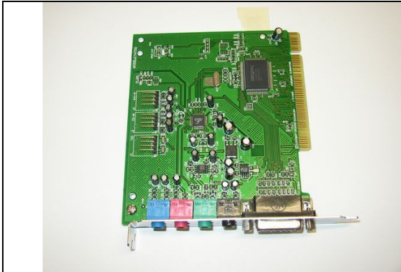
831.200.009 PC Sound Card Creative Lab 128 from System 32 (Max Fire V1.18 and Silverball V9.32)
