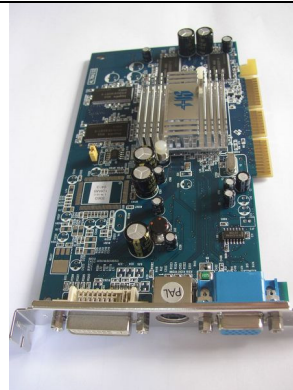
831.000.072 PC Grafikkarte ATI Radeon 9200 128MB DDR ab System 127 (Max Fire Video V1.01 und Virtual Pinball V1.12)
