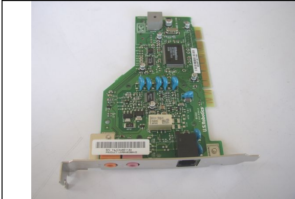
831.800.057 PC Modem PCI 56K 3com USRobotics from system 19 (SSilverball V7.08, Max Fire V1.01) and from system 122 (Max Fire Video V1.00, Virtual Pinball V1.10, Virtual Casino V1.07) and from System 306 (Silverball Centurio on Strato and Cosmo and Max Fire (Video) V1.21)
