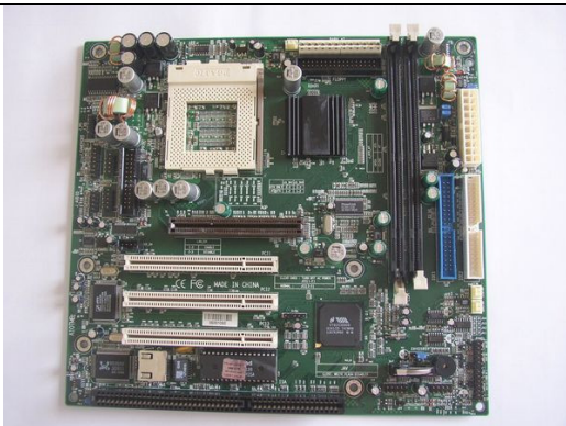
831.000.044 PC Motherboard QDI TAB from System 119 (Virtual Pinball V1.02, Max Fire Video V1.00)
