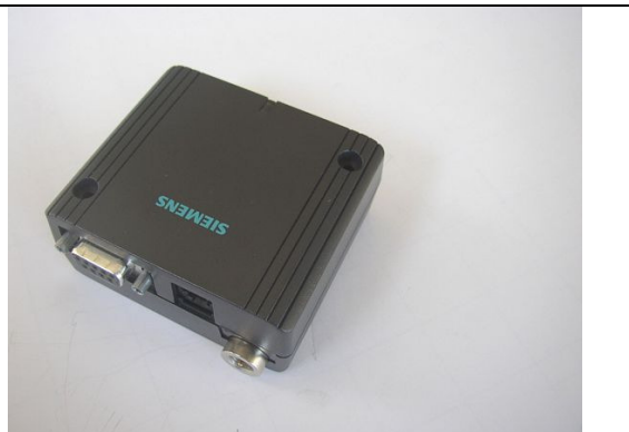
831.800.056 PC GPRS Modem Siemens MC35T from Silverball V7.04, Max Fire V1.00, Virtual Pinball V1.12, Virtual Casino V1.09
