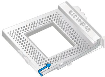
2. Align the blunt edge of the CPU with the matching pinhole on the socket.
