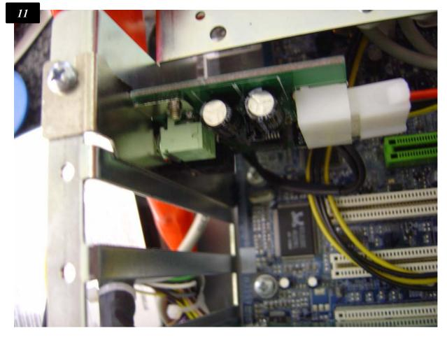
**Step 7:** The amplifier will be mounted in a slot (picture 11) and with the powercable connected. (picture 12).
