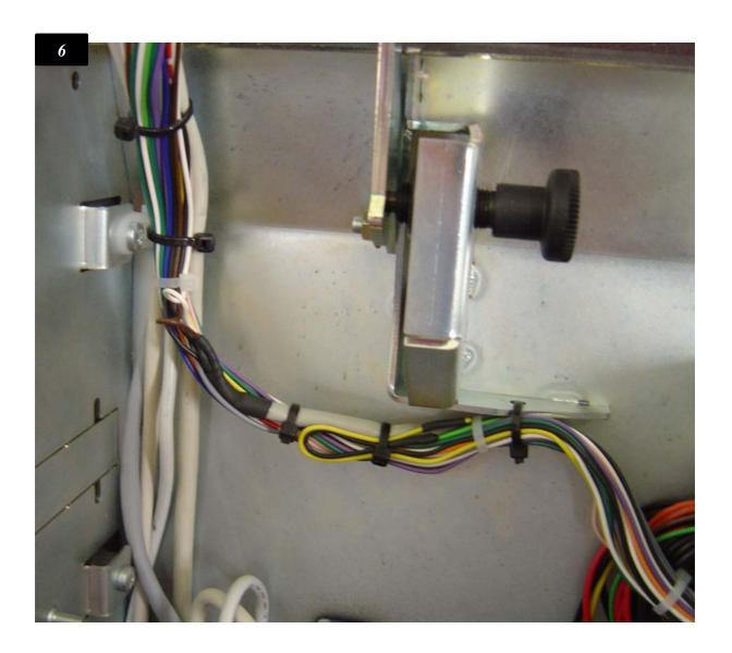
**Step 4:** Mount the reworked harness with binder in the machine. (picture 6)
