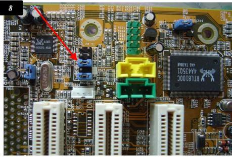
**Step 5:** Remove the jumper Gigabyte motherboard (picture 7) and PC Partner motherboards (picture 8).
