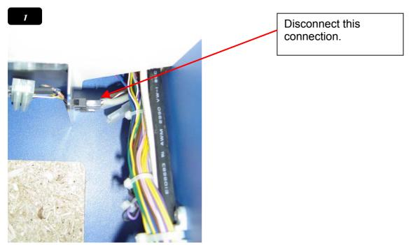
**Step 1:** Disconnect the connection to the two Kemo amplifier.
