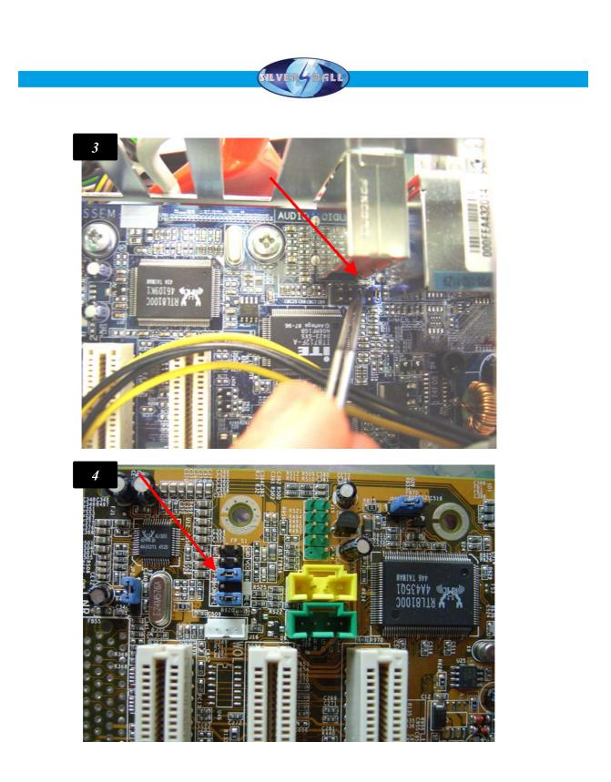
**Step 3:** Remove the jumper Gigabyte motherboard (picture 3) and PC Partner motherboards (picture 4).
